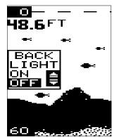
**NOTE:** Turning the unit off erases all user settings and it returns to the system defaults. For example, if you turn the lights on, then turn the unit off, the next time you turn the unit on, the lights will be off, since the default setting for the lights is off.
